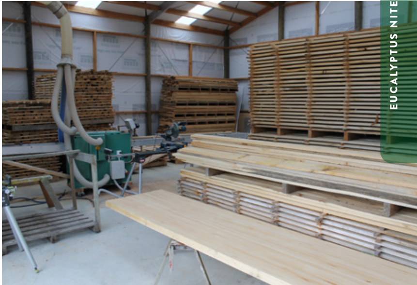
Above: Eucalyptus nitens being converted into flooring products, Specialty Timber Solutions, North Canterbury.
