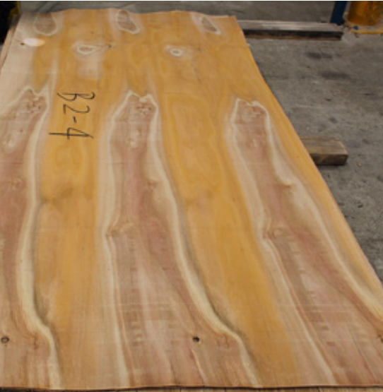
Left: Peeled E. bosistoana veneer – produced as part of NZDFI's wood quality research.
